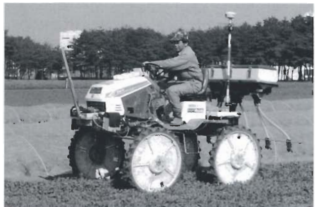
Precision Agriculture - A GPS controlled mobile carrier, NARO, Tsukuba
